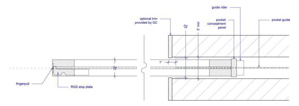
Guide rider is a block with a slit for the pocket guide; it allows for full extension, attach to bottom of concealment panel.
