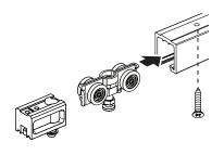
**4.** Drop bottom pivot point of panel into floor receiver.
