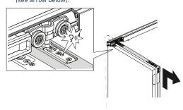
10. Test operation to ensure panels aren't binding. Adjust panel height as necessary. (see steps 6 and 9).
