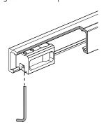
**5.** Push up plunger on top pivot in track and let it click into pivot receiver at top of panel.
