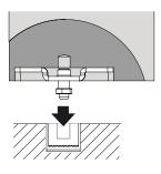
7. Lift second panel in pair and insert suspending bolt from wheel into top of panel. Pull until you hear a click. (see arrow below).
