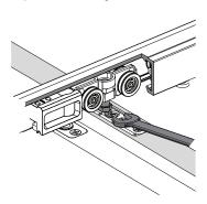
**12.** To install dust proof strike, mark on floor where flush bolt rod strikes. Drill floor with 11/16" drill bit and insert dust proof strike with a small amount of adhesive.
