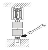
**9.** Adjust second panel height at top of door using wrench.
