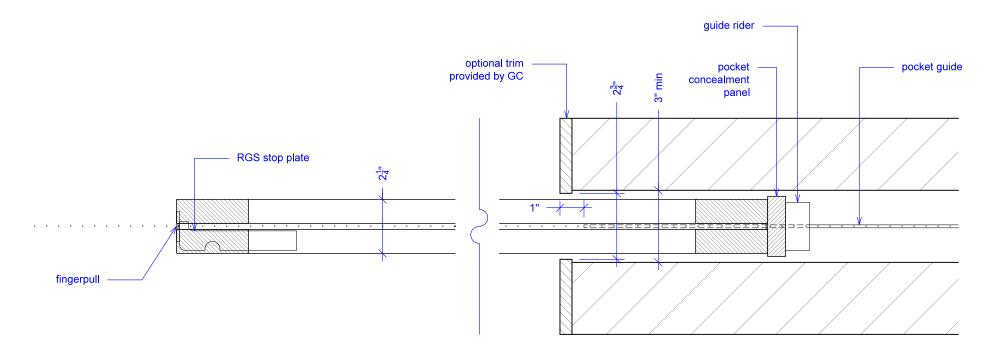
Guide rider is a block with a slit for the pocket guide; it allows for full extension, attach to bottom of concealment panel.
